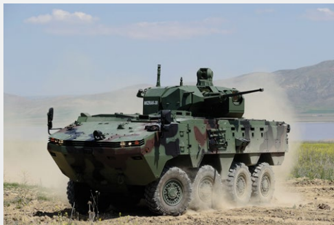
PERSONNEL CARRIER WITH MIZRAK 30 mm MEDIUM CALIBER REMOTE CONTROLLED TURRET
